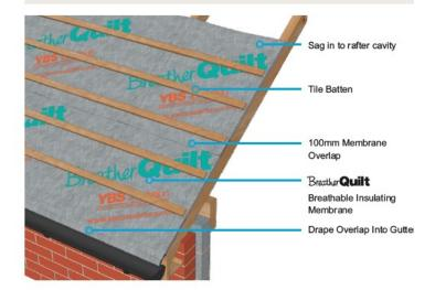
Starting at the edge of the roof and working horizontally, nail or staple BreatherQuilt to the irst rafter using 14mm staples, BreatherQuilt should hang down between the rafters ensuring once tile battens are installed a clear 10mm drape is formed at the centre of all rafter spaces.
