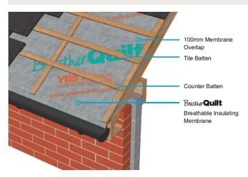
Starting at the edge of the roof and working horizontally, nail or staple BreatherQuilt to the irst rafter using 14mm staples, pull taught and proceed across the roof.
