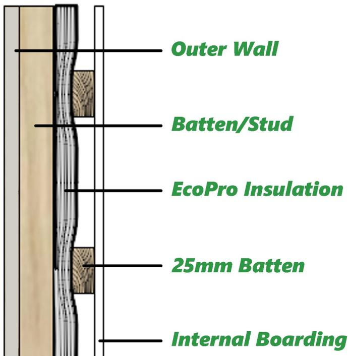
If Installing EcoPro onto the walls of your Static Caravan we would recommend the following;
