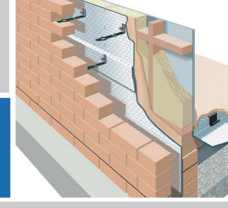
Specifically designed for timber frame and modular building applications.
