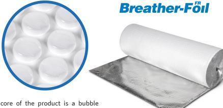
The core of the product is a bubble structure, formed using LDPE which contains an FR aditive. Each pocket of air offers high thermal performance and reduces the risk of cold bridging.
